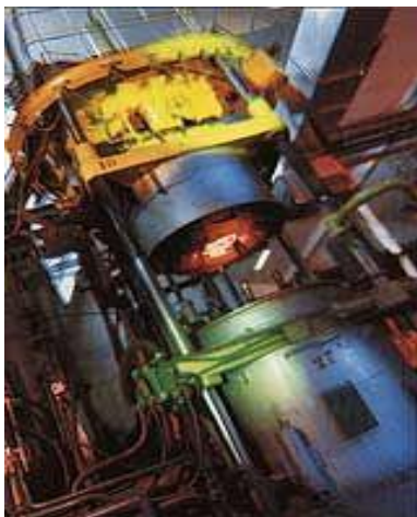
Back pressure casting technology facilitates the extremely precise and energy-conscious moulding of metal pressure parts made of aluminium. (Photo: Peter Allert)
