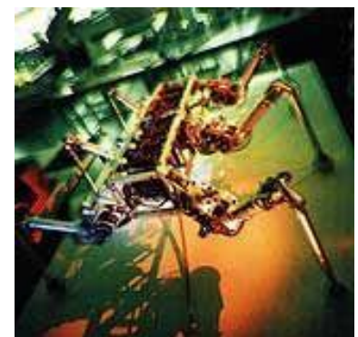
Using stick insects as examples, knowledge on the timing of neural stimuli is transferred to a robot model. (Photo: Friedrun Reinhold)
