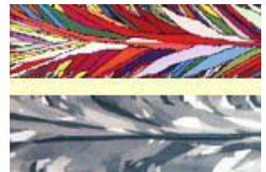
Simulation of grain structure in cooled metal (top) and section of metal rod cast under real conditions (bottom). (Photo: Friedrun Reinhold)
