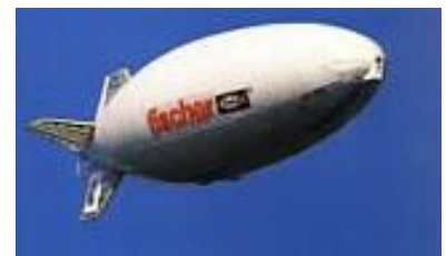
“Lotte”, the first solar powered airship, has been flying since 1993 and is the starting point for the development of the high-altitude platform. (Photo: Colin Barschel)
