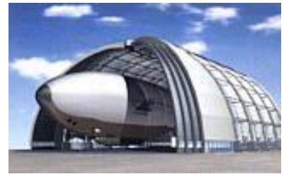
Heavy-duty transporters of the future: the 240 meter long CargoLifter is soon supposed to be able to carry up to 160 tons of cargo over long distances.
